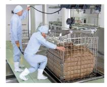
prescribed herbs are steeped and circulated in the wine base, and the active ingredients are extracted. As the speed of extraction differs according to the herb, this process requires a high level of skill and close management.
